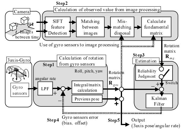
**Fig. 1.** System architecture of the proposed method.
