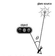
Fig. 4. Positional relationship between object and glare source
