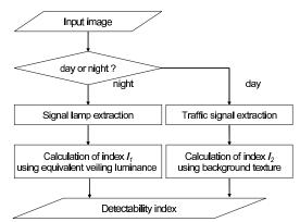
Fig. 2. Flowchart for calculating detectability index
