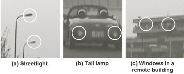
Figure 2. Objects whose characteristics resemble the image features of a raindrop.
