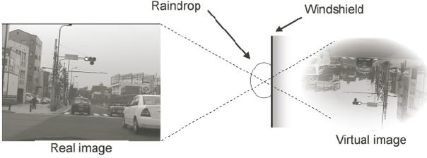
Figure 1. Image features of a raindrop.
