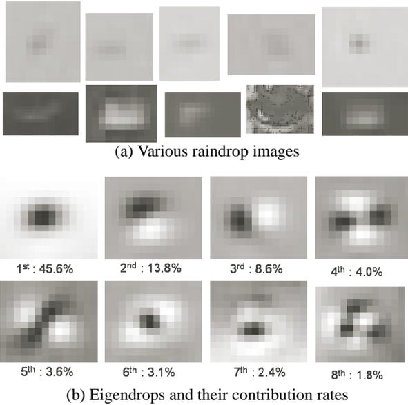
Figure 4. Examples of raindrop images and eigendrops.
