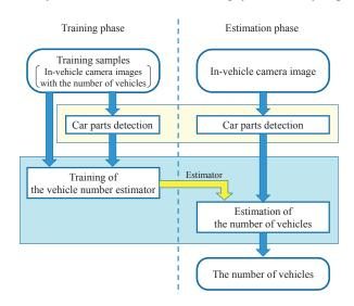
Fig. 2. Process-flow of the proposed method.
